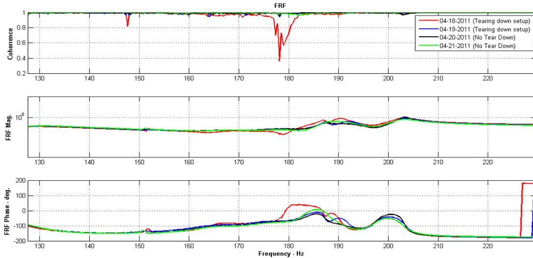
**Figure 10 - FRF Repeatability, Modal Shop Shaker, 130-230 Hz (Random input, 8192 Block size, 5 cyclic blocks, 37 averages, Hanning window, H1 estimation, Nyquist frequency 3000Hz)**
