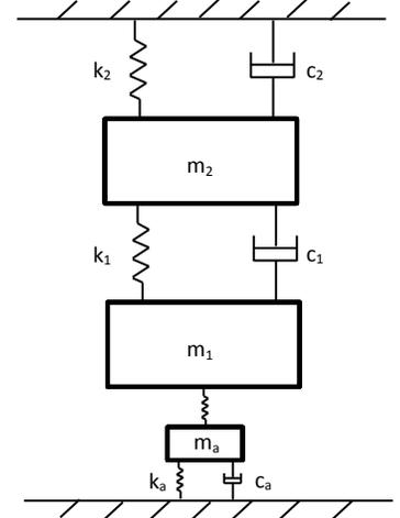
Figure 2 - 2DOF system excited by one shaker
