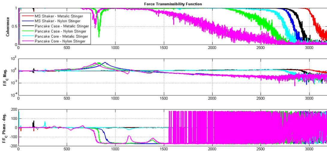
Figure 6 - Force transmissibility function, all shakers, different stinger material (Random input, 8192 Block size, 5 cyclic blocks, 37 averages, Hanning window, H1 estimation, Nyquist frequency 3000Hz)
