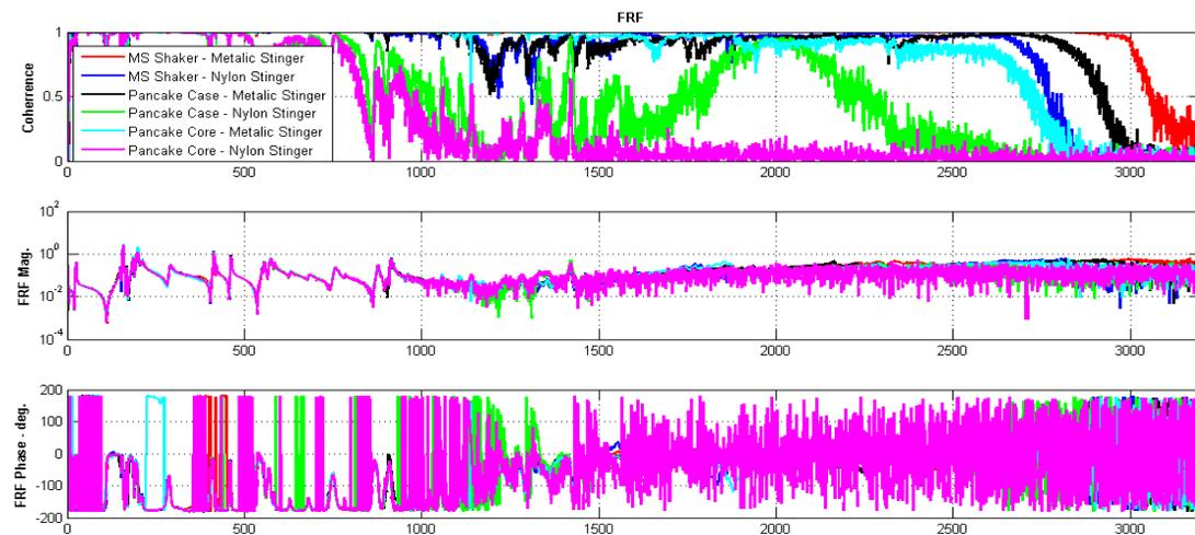
Figure 7 - Frequency Response Function, all shakers, different stinger material, 0-3000Hz (Random input, 8192 Block size, 5 cyclic blocks, 37 averages, Hanning window, H1 estimation, Nyquist frequency 3000Hz)
