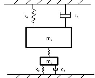
Figure 1 - SDOF system excited by one shaker
