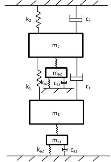
Figure 3 - 2DOF system excited by two shakers
