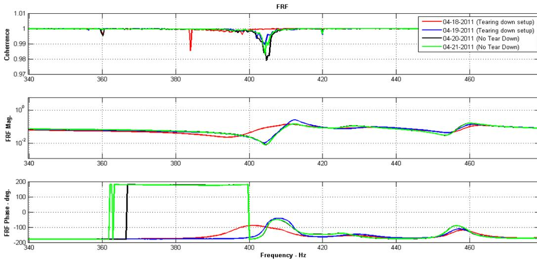
**Figure 11 - FRF Repeatability, Modal Shop Shaker, 340-480 Hz (Random input, 8192 Block size, 5 cyclic blocks, 37 averages, Hanning window, H1 estimation, Nyquist frequency 3000Hz)**
