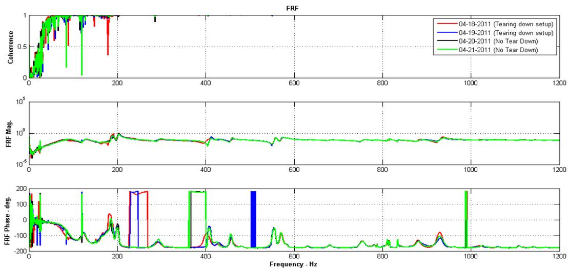
**Figure 9 - FRF Repeatability, Modal Shop Shaker, 0-1200 Hz (Random input, 8192 Block size, 5 cyclic blocks, 37 averages, Hanning window, H1 estimation, Nyquist frequency 3000Hz)**
