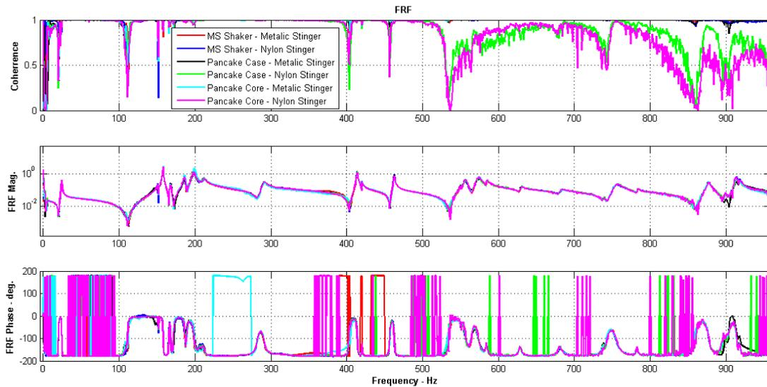
**Figure 8 - Frequency Response Function, all shakers, different stinger material , 0-1000Hz (Random input, 8192 Block size, 5 cyclic blocks, 37 averages, Hanning window, H1 estimation, Nyquist frequency 3000Hz)**
