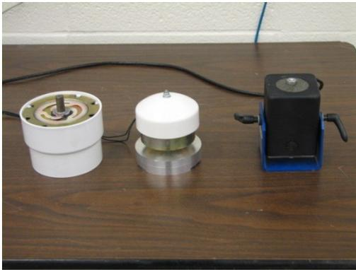
Figure 4 - Shakers from left to right Pancake-Core, Pancake-Case, and PCB 2004E
