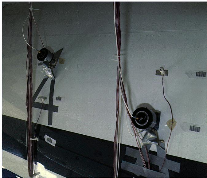
**Figure 9** – Structcel and Impedance Head Exciter Installation Spatial Sine Testing Setup
