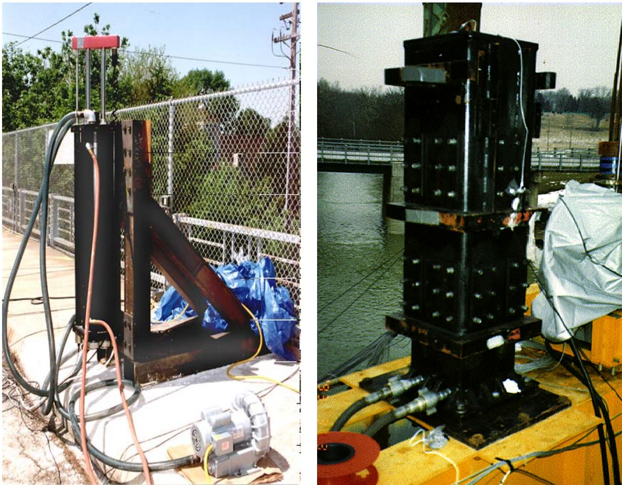
**Figure 10** – Electro-Mechanical Exciter - (Left) and Hydraulic (Right)
