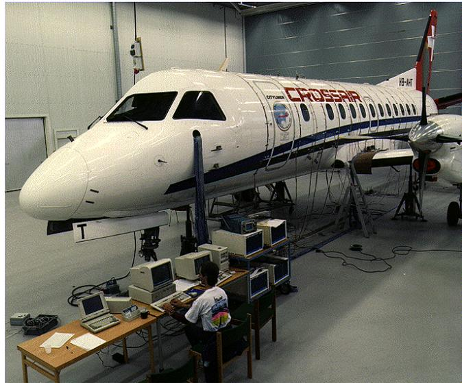
**Figure 8** – Saab Aircraft Spatial Sine Test
