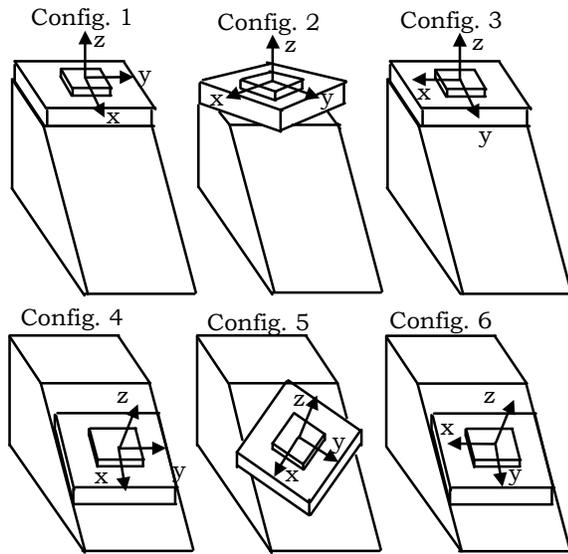
**Figure 4:** 6 test configurations of the load cell and rigid body mass.
