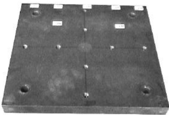
**Figure 9:** Single steel plate used as sub-structure.
