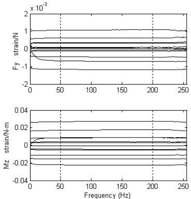
**Figure 5:** Sample force and moment calibration curves of the ICP strain gage 6-DOF load cell.
