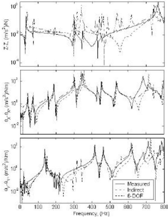
**Figure 14:** Driving point impedance model and physical measurement results for z-axis translation and x-axis and y-axis rotations.
