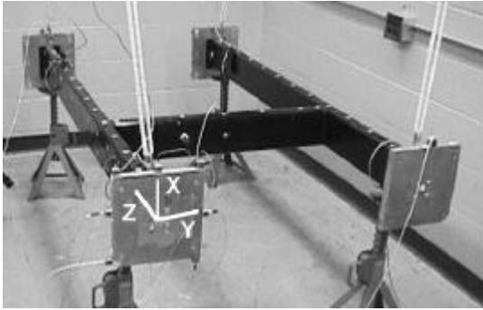
**Figure 8:** Baseline H-frame with aluminum endplates.
