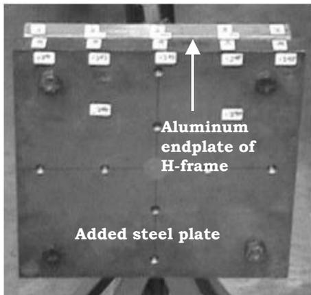
**Figure 12:** Physically modified H-frame with steel plate added to aluminum endplate.
