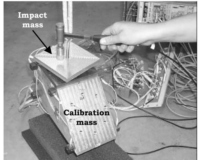
**Figure 3:** Load cell with impact mass and rigid body calibration mass.
