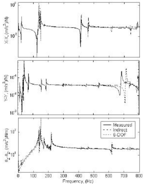
**Figure 13:** Driving point impedance model and physical measurement results for x-axis and y-axis translations and z-axis rotation.
