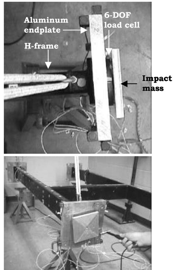
**Figure 10:** Impedance measurements on baseline H-frame using calibrated 6-DOF load cell.
