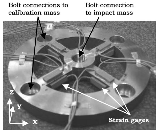
**Figure 1:** ICP strain gage placement on 6-DOF load cell.
