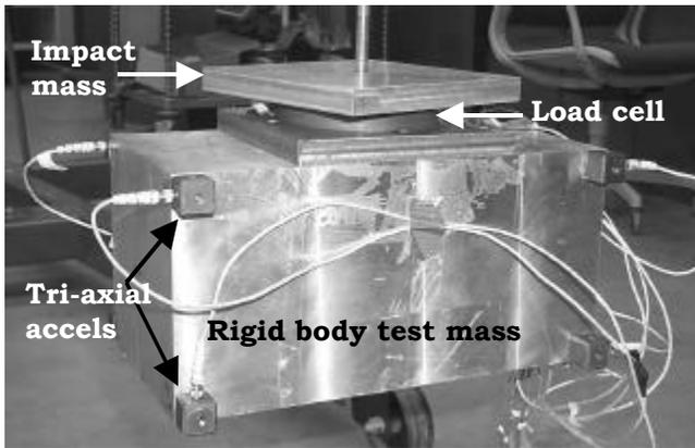
**Figure 6:** Rigid body mass used for inertia estimation.
