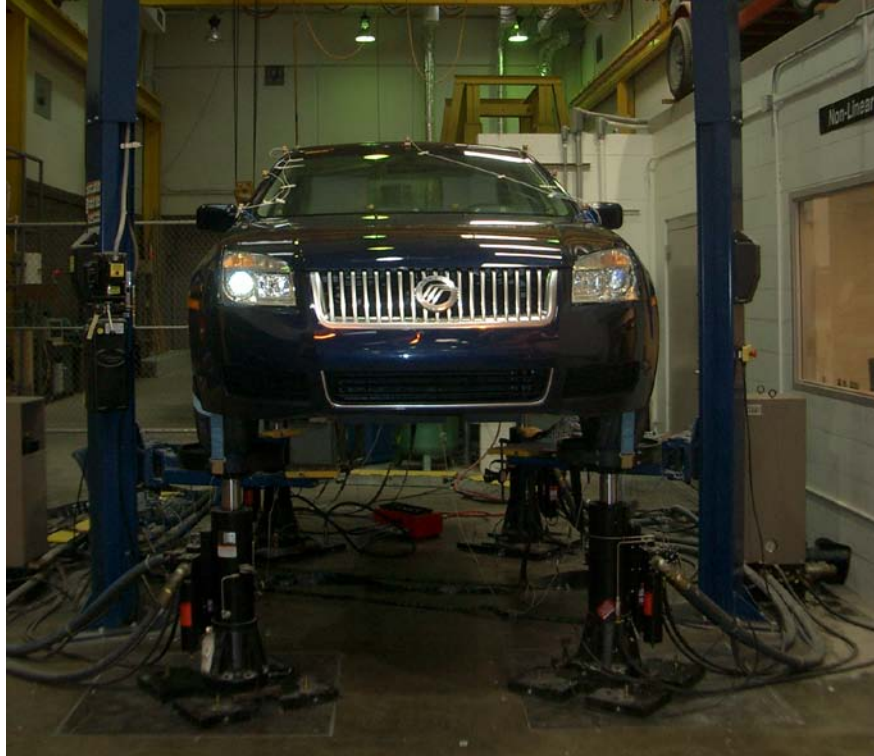
Figure 3-1 Typical Four Poster Shaker Setup
