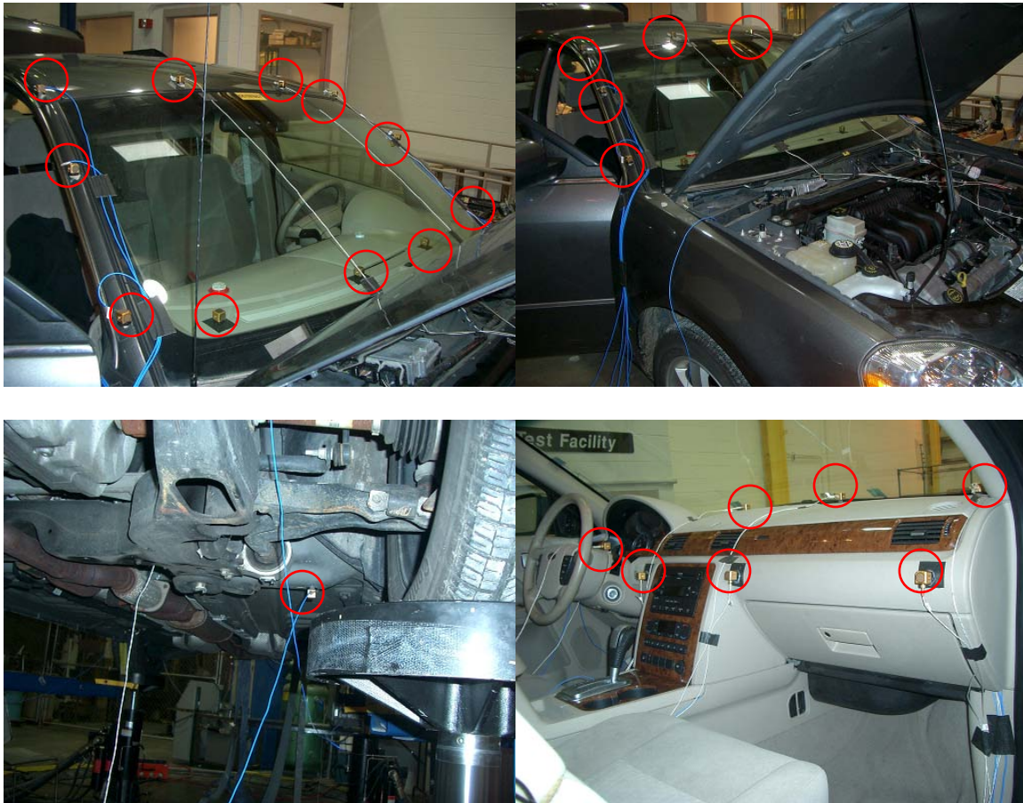
Figure 3-3 Various Locations of Accelerometers on the Vehicles
