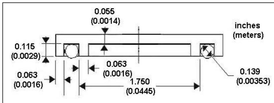
**Figure 13. Design Adjusted for Standard Seal**
