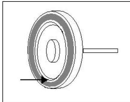
**Figure 27. Simply Supported Boundary Condition Constraint Location**
