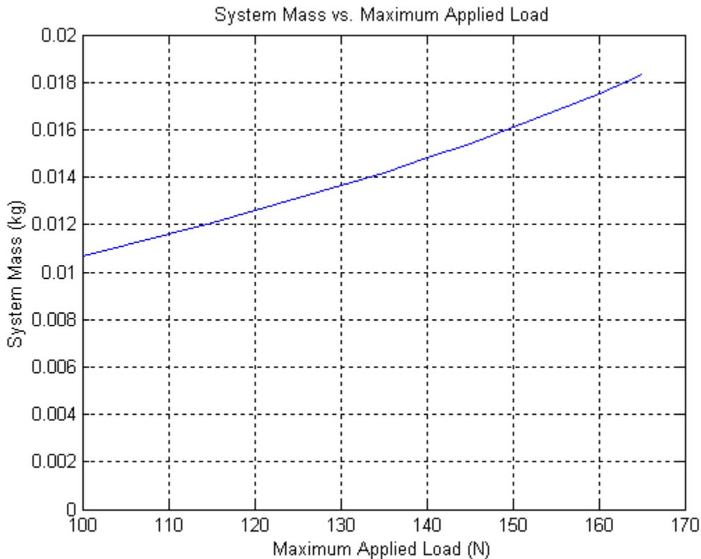
**Figure 11. Design Sensitivity to Maximum Applied Load.**
