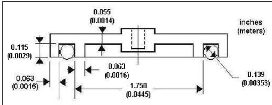
**Figure 14. Adjusted Fixture Geometry for Threaded Attachment**
