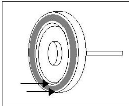
**Figure 24. Mounting Surface of Attachment Fixture**
