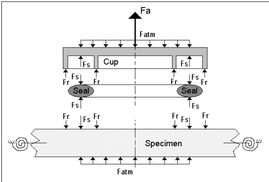
Figure 2. Generalized Loading Condition of the Attachment Fixture
