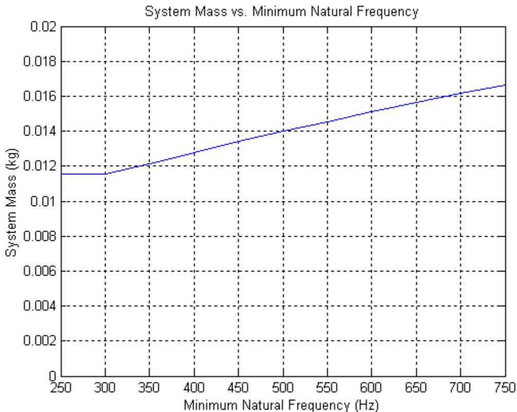
**Figure 12. Design Sensitivity to Minimum Natural Frequency**
