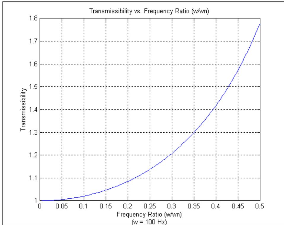
**Figure 7. Transmissibility vs. Frequency Ratio**
