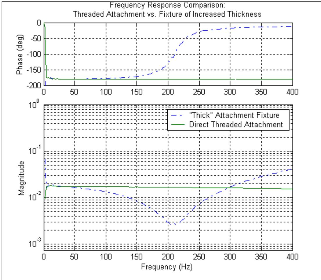
**Figure 22. Response Comparison of Threaded Attachment and “Thick” Fixture**
