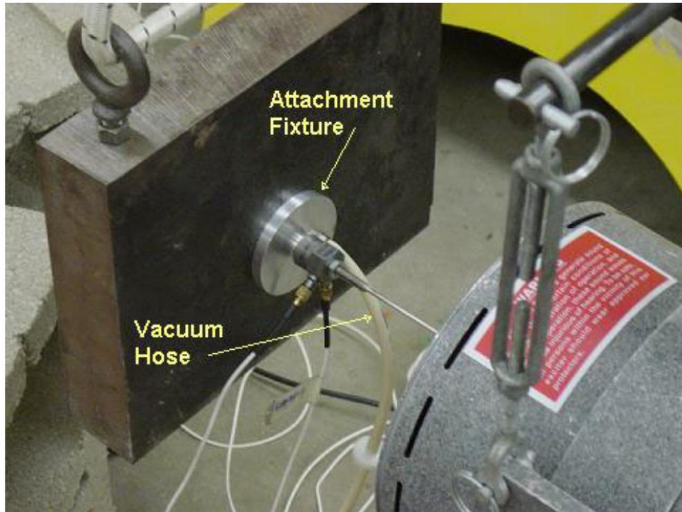
**Figure 18. Pneumatic Attachment Fixture**
