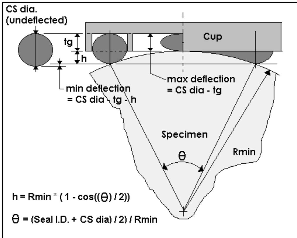
**Figure 5. Curved Mounting Condition Geometry Considerations**
