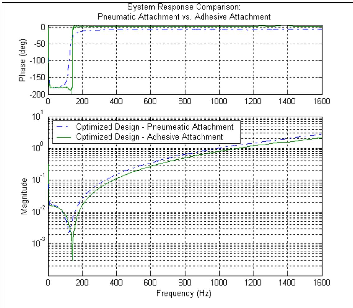
**Figure 23. Comparison of Adhesive Attachment and Pneumatic Attachment**
