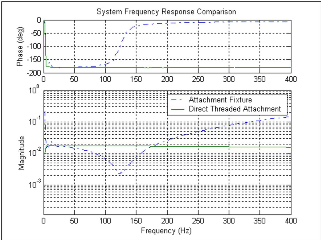
**Figure 20. Comparison of Connection Method Performance**
