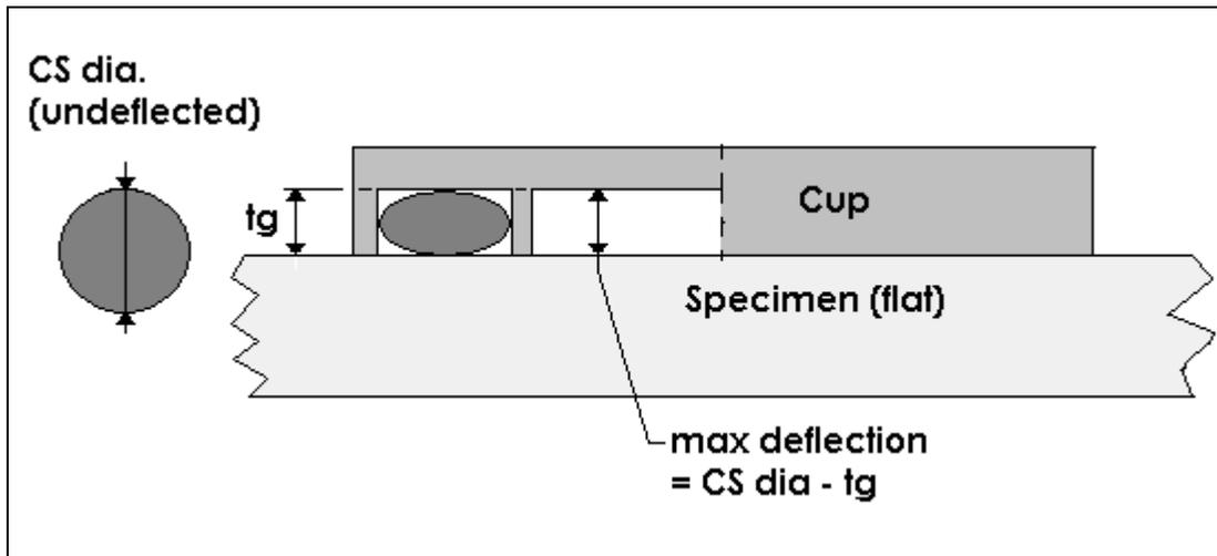
**Figure 4. Flat Mounting Condition Diagram**
