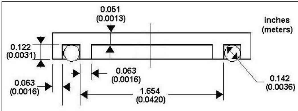
**Figure 10. Optimized Solution of Attachment Fixture**
