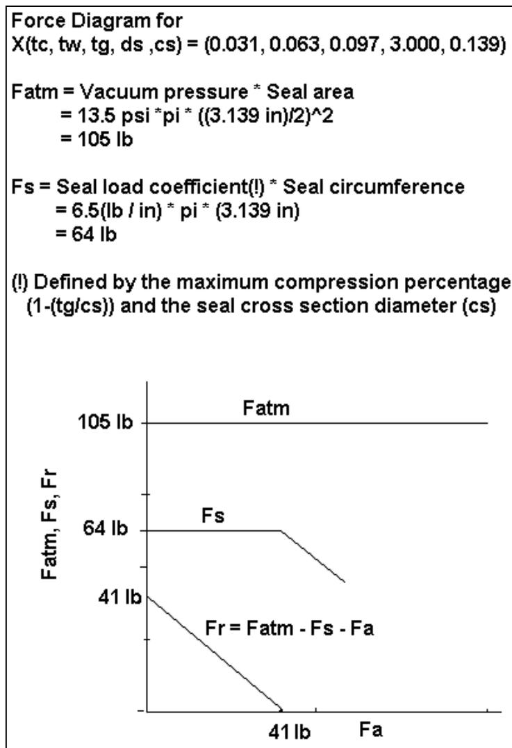
**Figure 3. Force Diagram for Arbitrarily Chosen Design Vector**
