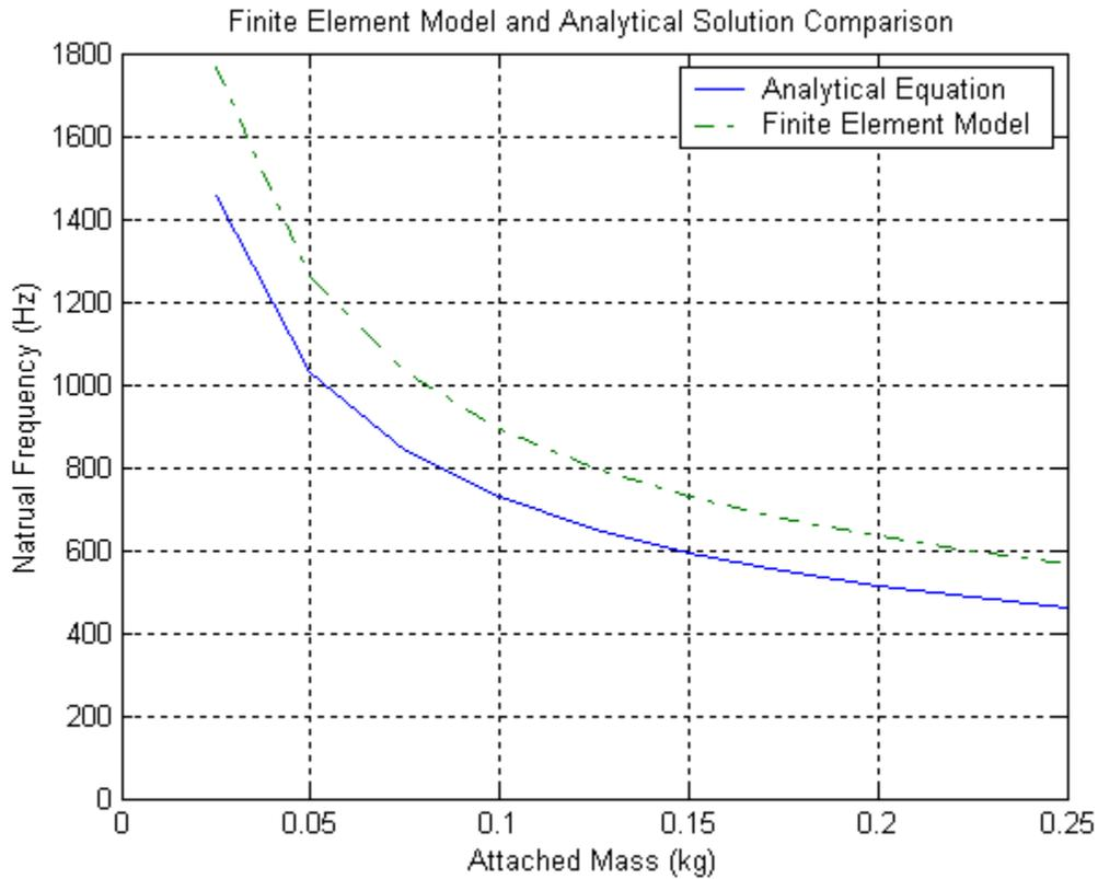
**Figure 25. Finite Element Model and Analytical Solution Comparison**
