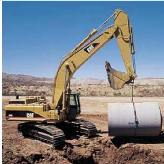
**Figure 1-1: Caterpillar Hydraulic Excavator using hydraulic controls to position a large section of piping. (Courtesy of [www.cat.com](http://www.cat.com))**
