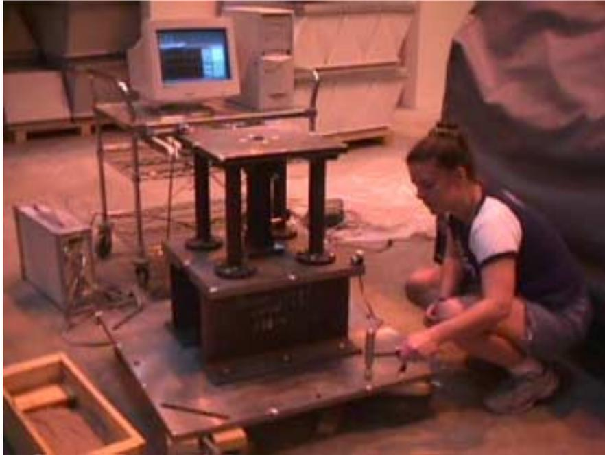
Figure 5-5: The vibrations test set up with the 2 ½" cylinder in place in the stand.
